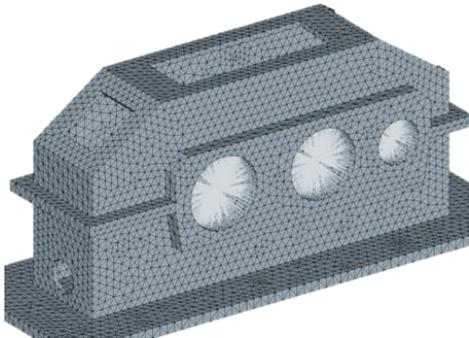
It is now also possible to use the damage data for all elements when performing a strength analysis for the entire gear unit or drive train. This enables the weakest element in the drive train to be identified quickly and easily, so that the user can make the necessary design changes immediately.
