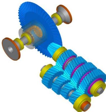
KISSsoft calculates the service life and strength of the different machine elements, and transfers the results to KISSsys, where they are displayed in clear overviews. To achieve this, KISSsys brings together kinematic analysis, service life calculation, 3D graphics, and user-defined tables and dialogs.
