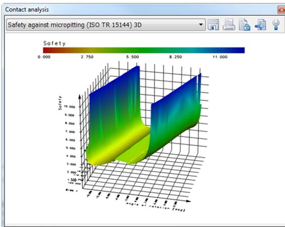
In theory, micropitting will not occur if the lubricant film is thick enough. The permissible specific lubricant film thickness depends on which lubricant is used, in particular which additives are involved, the surface structure, and other parameters such as the hardening process.
