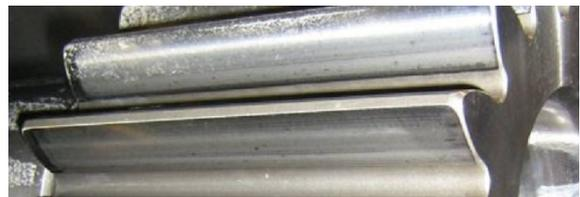
The removal of material from the flank increases the profile error of the tothing and therefore leads to a general reduction of its quality and precision. After a time, the material removal may stop or this process can continue.
